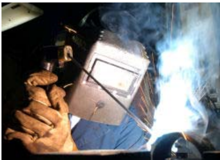
Manual arc welding
