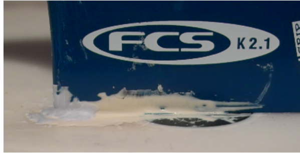
Surf board fin repaired with epoxy resin
