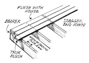
Check every fifth or sixth board to ensure they are still parallel with the house foundation and that the outside ends of the boards overhang the outside joists.
