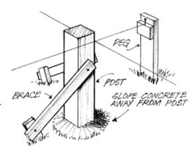
Align the outside edges of the pile with the string lines. If necessary, provide temporary braces to the pile to secure it in position while concrete is placed in the hole.
