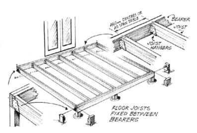
Trim the front edge of the joists 50mm inside the outside string line.
