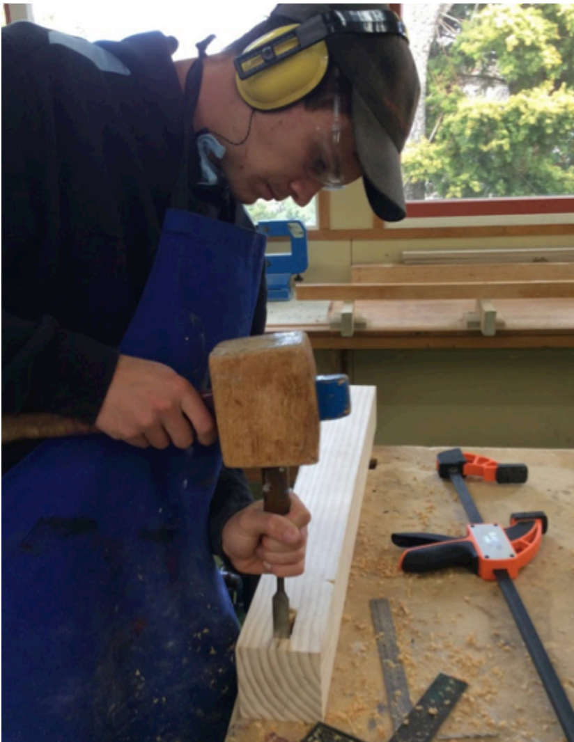
Chiselling out the mortise.
