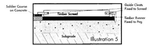
Screed the sand to a uniform level. When screeding, guides or runners are needed on each side to run the screed board on. If there is already a soldier or kerb course of pavers for edging in place, this can be used to support the runners. If not, drive pegs and fix runners to them, just like concrete boxing.
