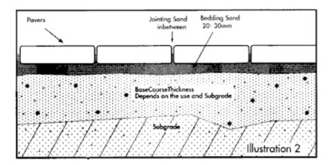
Quantities of base course material and bedding sand are calculated in volume of cubic metres (m³) – length x width x depth. (You also need to allow a bulking factor for bedding sand and base course material so that you achieve correct depth once they are compacted. The supplier can tell you what percentage to allow.)
