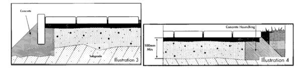
Existing pathways, or other permanent structures (such as house foundations), can be used to retain both the bedding sand and pavers. For many projects other methods of edge restraint must be used to ensure the paved area remains level.
