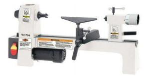
Never wear ties, rings, long hair or loose clothing when using a lathe.
