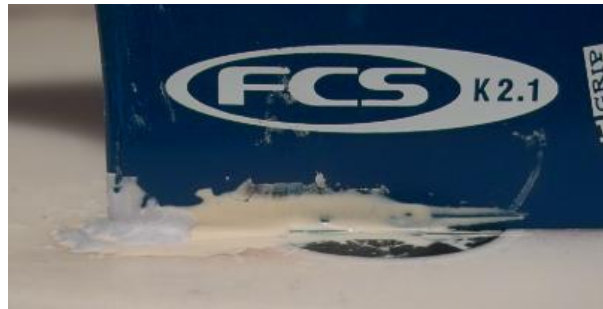
Surf board fin repaired with epoxy resin
