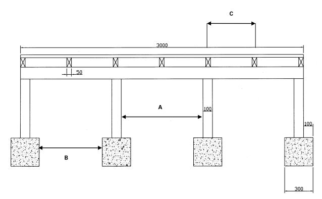
a) A deck needs to be constructed. (See sketch above.) The length of the deck is 3 metres. The foundation piles are 100 x 100 H4 radiata pine mounted in 300 x 300 concrete footings. Four are to be evenly spaced along its length. Calculate the spacings (Distance A on the sketch).
