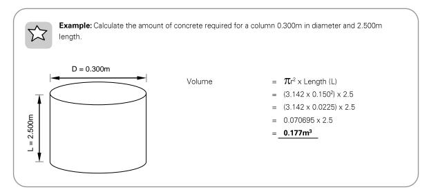
Another way of approaching the concept of volume is to consider that it is the cross-section area x length (or height, depending on its application).
