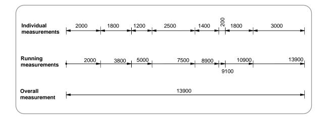
Dimensions on working drawings are usually shown as individual and overall measurements. When running measurements are required, then the dimensions will need to be added together.
