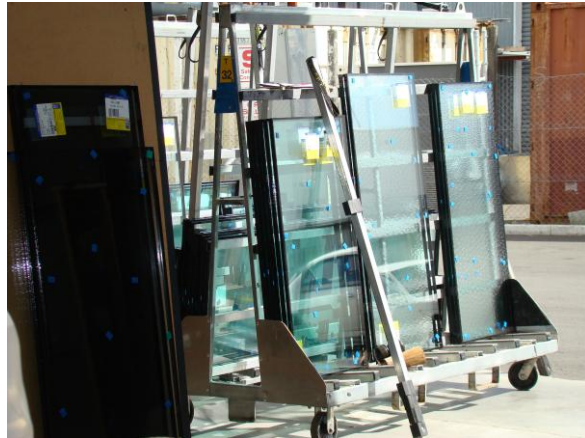
IGU panels made to size are ready to be assembled into joinery units.
