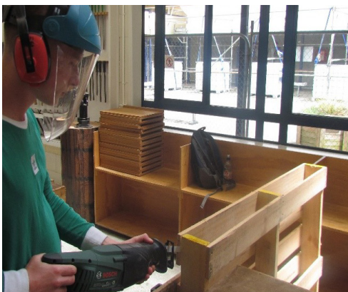
Careful use of sabre saw (left) and hacksaw (right) to cut through nails
