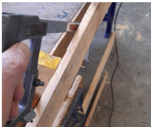
Careful use of sabre saw (left) and hacksaw (right) to cut through nails
