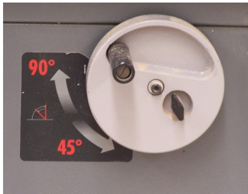
Set your machines up before beginning work
