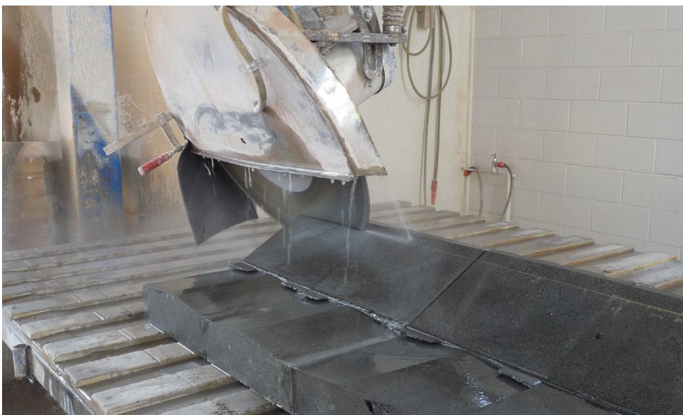
Masonry table saws can cut stone precisely and with little vibration.
