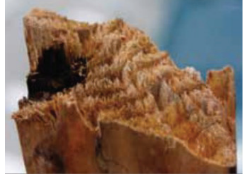
Fracture surface of timber with soft rot.
