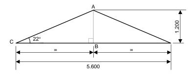
2. Using Pythagoras theorem, calculate the length of the rafter A - C.
